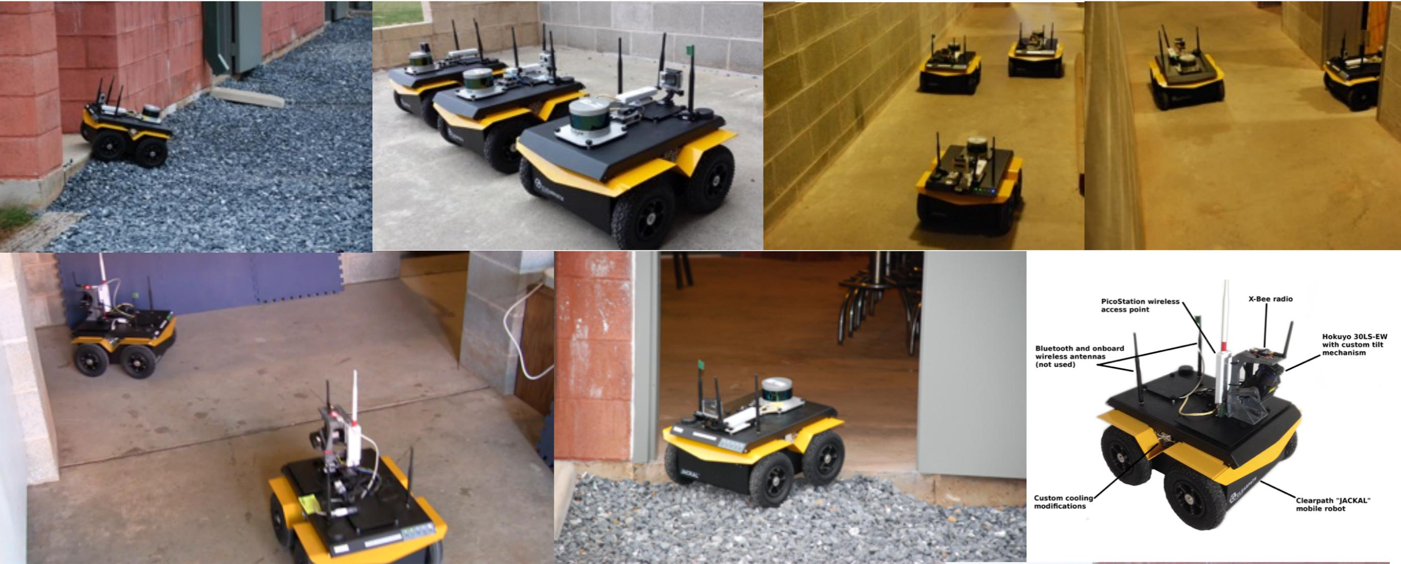
We tested the proposed approach on field data collected by two to four Jackal robots, moving in a military test facility. We use the estimated trajectories to reconstruct a 3D map of the facility.
