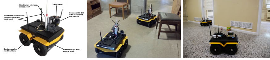
Figure 39: (Left) Clearpath Jackal robot used for the field tests: platform and sensor layout; (right) snapshot of the test facility and the Jackal robots.
