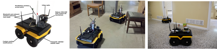
Fig. 6. (Left) Clearpath Jackal robot used for the field tests: platform and sensor layout; (right) snapshot of the test facility and the Jackal robots.
