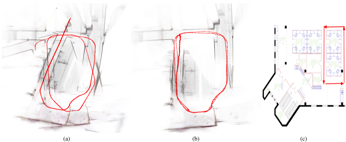
Fig. 8: Trajectories estimated with and without using objects as landmarks during loop closure. (a) Robot trajectory estimated when using no object landmarks. (b) Robot trajectory estimated when using object landmarks for loop closure. (c) Shows the approximate ground truth trajectory w.r.t the floor plan.
