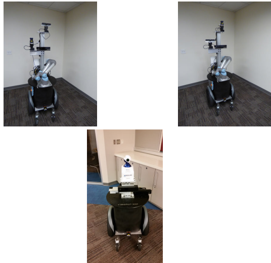
Fig. 6: The figures above show an example reconfiguration for the experiments conducted. The figure on the top left shows the Hokuyo laser on the top of the robot and the figure on the top right shows the Hokuyo laser towards the right of the robot. The figure on the bottom shows another possible configuration of the robot mounted with two Kinect sensors, a Roboteye RE05 and a Hokuyo laser.
